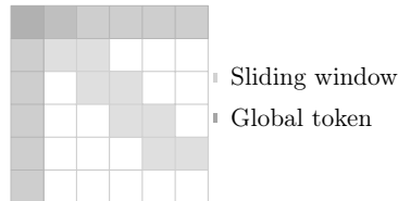
Figure 4: Schematic attention mask used by Longformer, combining a fixed-width sliding window (light grey diagonal band) with global tokens that attend to, and are attended by, all positions in the sequence (dark grey row and column). Diagram redrawn after Beltagy, Peters, and Cohan [BPC20].
