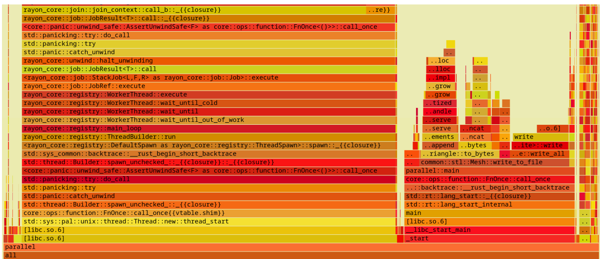
Figure A.4: Excerpt from the flamegraph of the parallel Rust version. Generated using [31]
