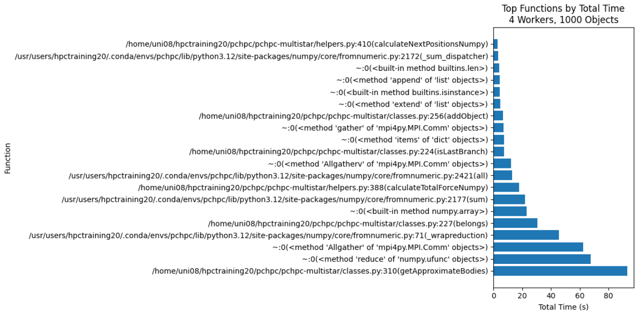
Figure 17: cProfile of simulation with 1000 objects in parallel with 4 workers. The values are averaged by number of workers. After the optimization.
