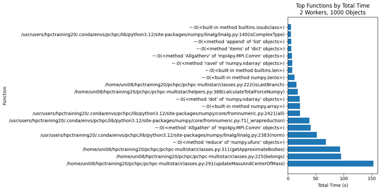
Figure 15: cProfile of simulation with 1000 objects in parallel with 2 workers. The values are averaged by number of workers. Before the optimization.
