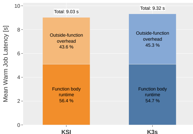
Per stack ( KSI/K3s ): mean over n = 320 successful invocations ( 5 \text{ runs} \times 64 \text{ Jobs} ) in the warm two-node benchmark setup. The mean is used so that the stacked bars decompose total warm Job latency exactly and the percentage shares sum to 100 %.
