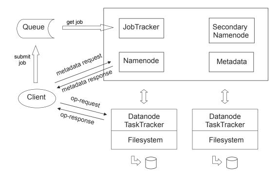
HDFS has a client/server architecture. A HDFS cluster consists of two masters: Namenode and JobTracker, multiple Datanodes and is acessed by many clients.
