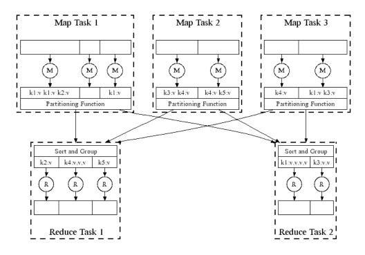
The above graphic shows that an input data set is split into three split sets which are committed to the map tasks and each map task runs on a different node. For example the map task "*I*" handles the 1st split data set containing 3 files and calls one map function for each file.
