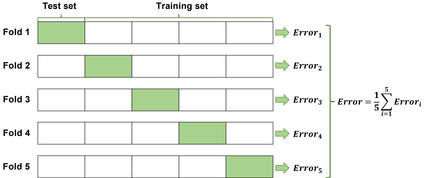
The principle of 5-fold cross-validation
